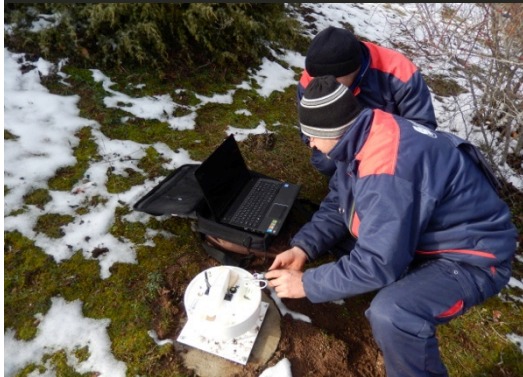
“Gauges with internal data loggers have been installed to collect precipitation data at specific points around our project site” – Dragi Peltechki, Mining Engineer
