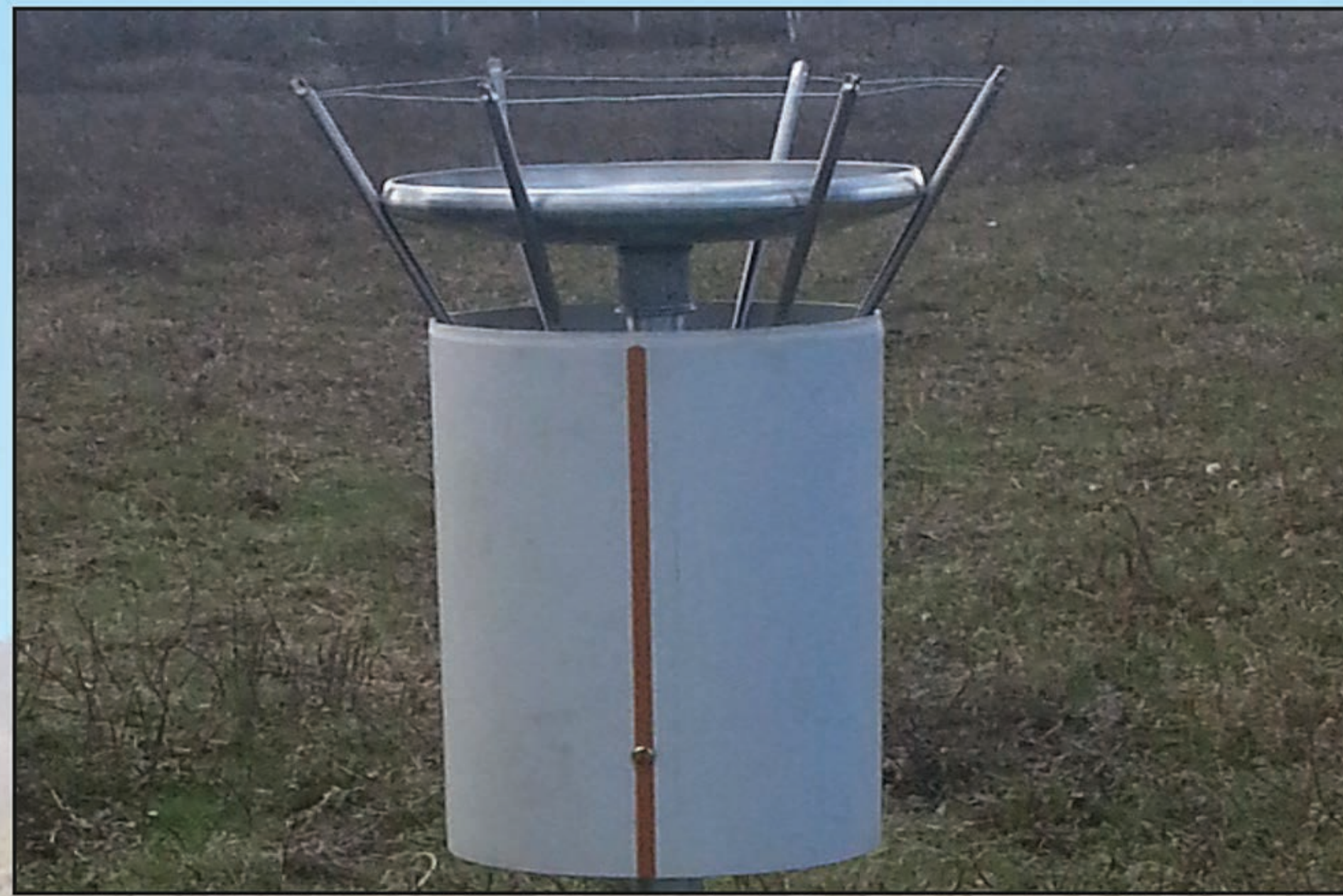
Frisbee gauge Deposited dust
