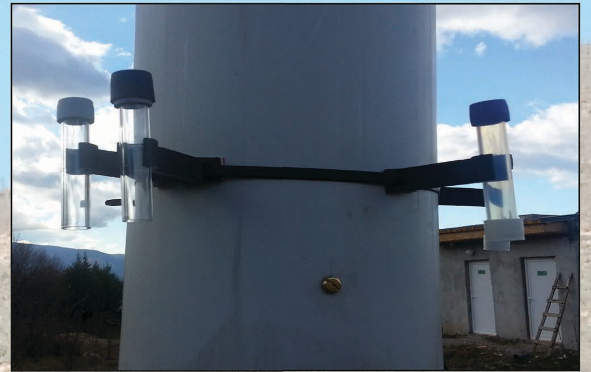
Diffusion tubes NO, NO 2 , SO 2 and O 3
