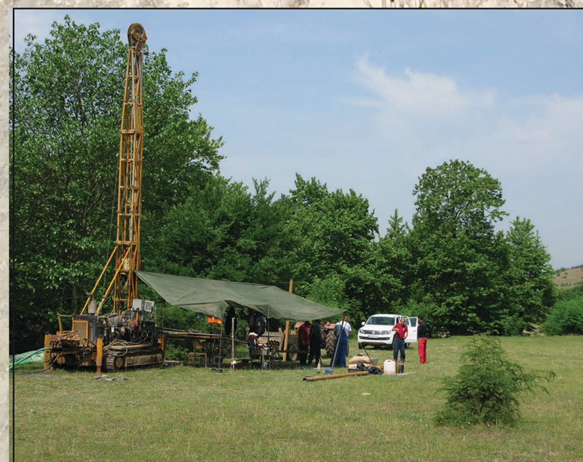
Installing piezometers for measuring groundwater levels
