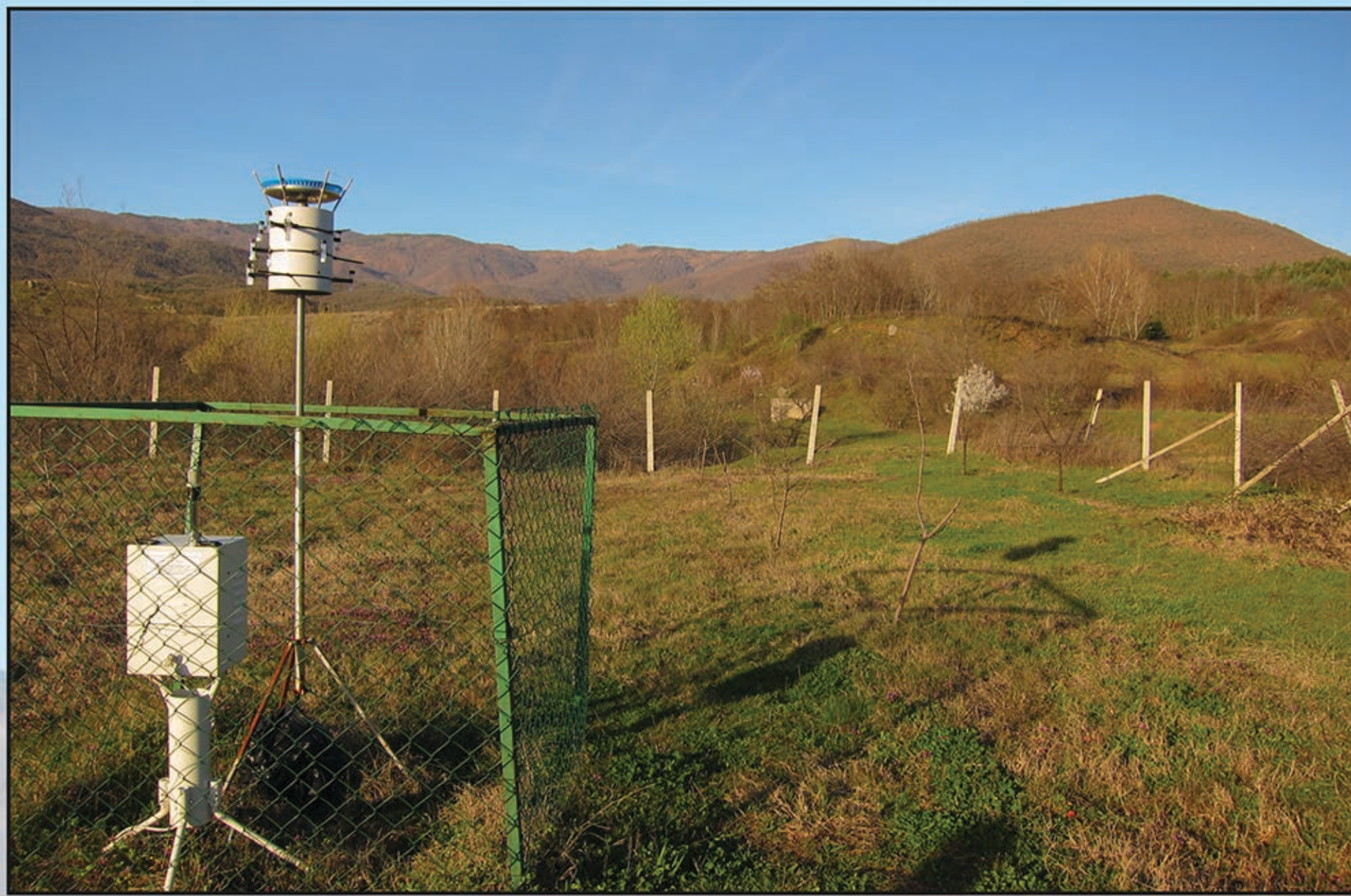
Osiris particulate monitor Monitored fine particulates (PM10, PM2.5)
